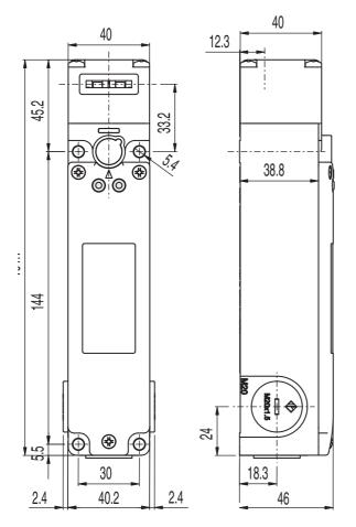
Figure 13.2: Dimensions of L200-M1C3-MLM24-L2G in mm
