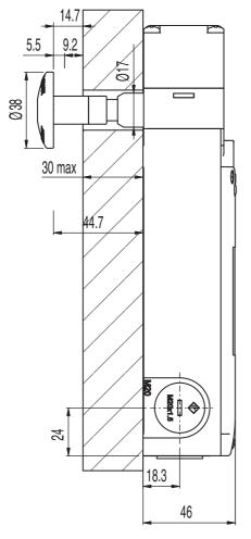
Figure 13.4: Dimensions of L200-M1C3-SLM24-PB-L2G in mm
