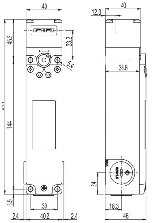
Figure 13.1: Dimensions of L200-M1C3-SLM24-L2G in mm
