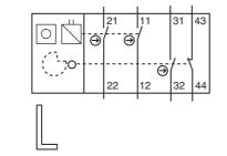
Figure 7.1: Contact block 3NC + 1NO (L200-M1C3-SLM24-PB-L2G, L200-M1C3-SLM24-L2G, L200-M1C3-MLM24-L2G)
