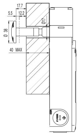
Figure 13.5: Dimensions of AC-PB40-L200 in mm
