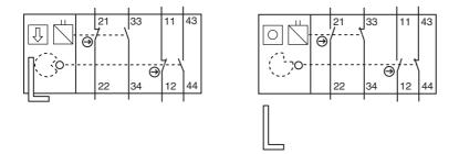
Figure 7.2: Contact block 2NC + 2NO (L200-M0C3-SLM24-L2G)
