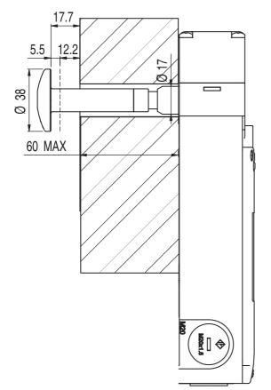
Figure 13.6: Dimensions of AC-PB60-L200 in mm
