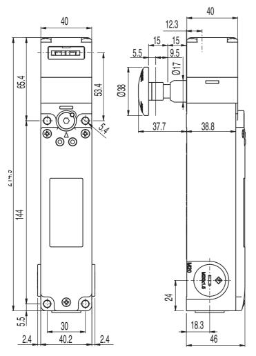
Figure 13.3: Dimensions of L200-M1C3-SLM24-PB-L2G in mm
