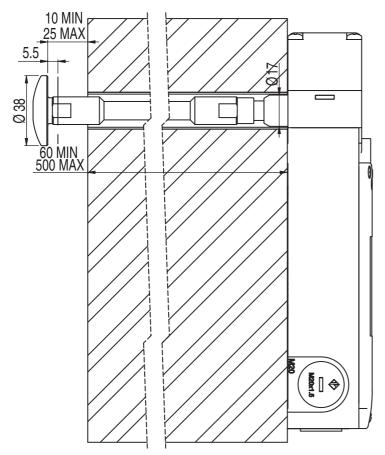
Figure 13.7: Dimensions of AC-PB500-L200 in mm
