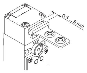
Secure actuator with rivets or tamperproof screws so that it cannot be detached.
