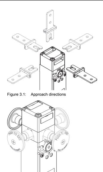
Figure 3.2: Actuation directions of the emergency release button
