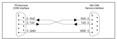
Figure 4.3: Connecting the service interface to a PC/terminal
