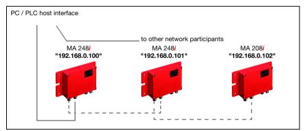
Figure 4.5: PROFINET-IO in a linear topology
