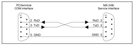
Figure 7.7: Connecting the service interface to a PC/terminal
