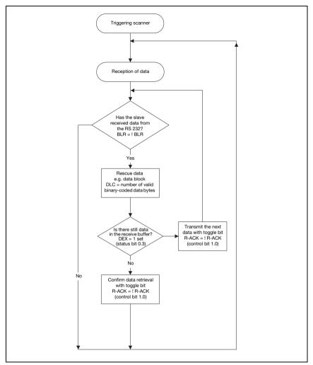
Triggering the ident devices and reading the data
