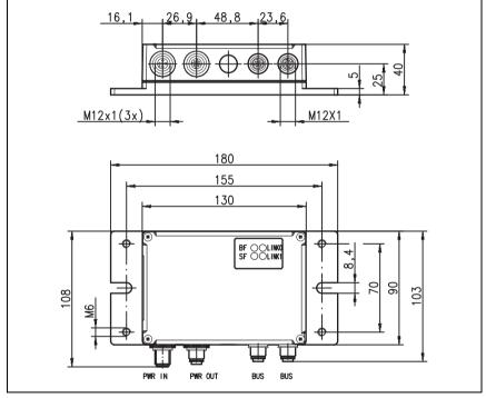
Figure 5.1: MA 248*i* dimensioned drawing
