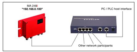
Figure 4.4: PROFINET-IO in a star topology
