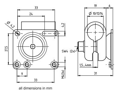
Fig. 12.3: Dimensioned drawing mounting system BTU 300M-D10/D12/D14
