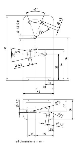
Fig. 12.4: Dimensioned drawing mounting bracket BT 300M.5
