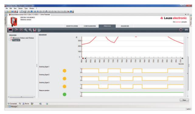
Fig. 8.11: PROCESS function – display of the measurement values
