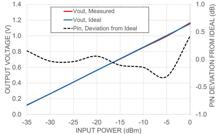
INPUT POWER DEVIATION FROM IDEAL vs INPUT POWER @ FREQUENCY 30 GHz
