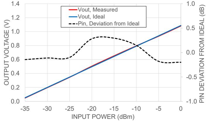
INPUT POWER DEVIATION FROM IDEAL vs INPUT POWER @ FREQUENCY 10 GHz
